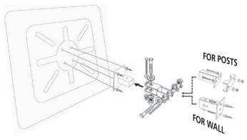
All mirrors are supplied complete with bolts and brackets kit in galvanised steel, adaptable for walls and round posts (Ø 76 to 90 mm) or rectangular (60x80 or 80x80mm).
